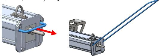
Grip the stainless-steel pull handle firmly and pull towards you. In the case where there is lots of debris collected, you may need to first pull swiftly to get the sleeve started off the magnet housing. It should get easier the further you pull the sleeve off.
