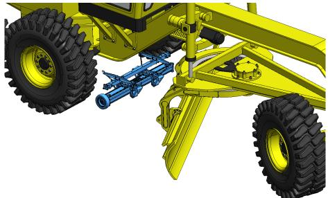
Note: The bump wheels on the ends of the sweeper should no less than 1/2"-1" off the ground when on level ground. The bump wheels on the sweeper will help to prevent ground strikes to the magnet housing and quick clean off sleeve. If you notice that the wheels on the ends of the sweeper are rolling on the ground frequently, it is recommended to raise the sweeper to prevent damage to the aluminum quick clean off sleeve.
